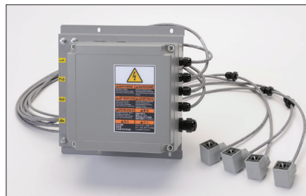
Sequencer box prioritizes the melter fill signal so that adhesive is added to only one melter at a time
